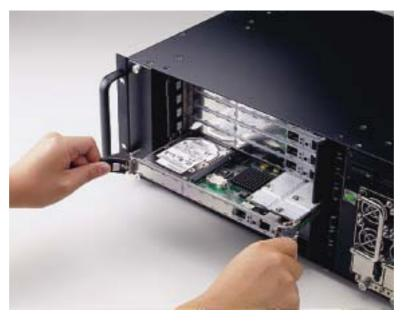
Figure 2-1: Installing the card into the chassis
